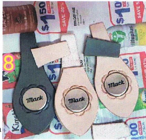
Photo (8); One end of the two part are cut off. And after the keyring is on place is the one left turned in and sewed
